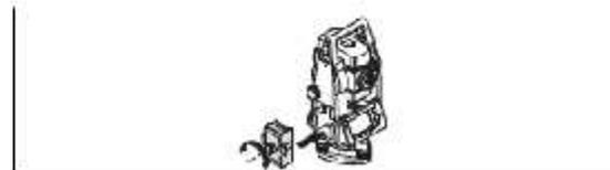
4. Insert battery holder into the instrument.
