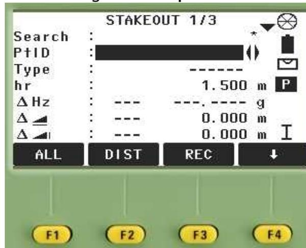
33. Now Move the Instrument until Hz equal to zero.
